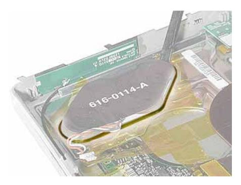
7. Install the replacement backup battery, and reassemble and test the computer.
