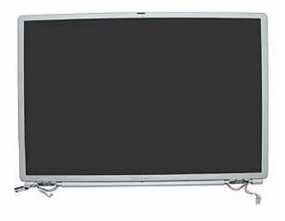
14. Install the replacement display module, and reassemble and test the computer.
