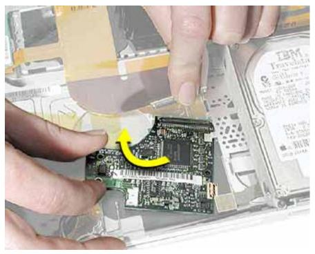
5. Install the replacement PMU card, and reassemble and test the computer.
