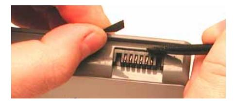
4. Use the stick to press the shim down and into place so it is centered and flush with the battery connector.
