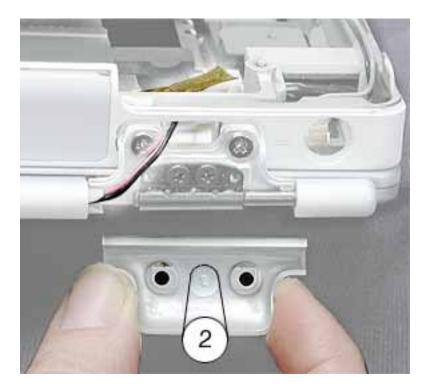
4. Warning: Be especially careful when working near cables that attach to the display. If any of these cables are damaged, the entire display module must be replaced.
