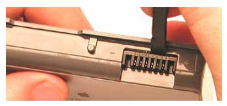
**Note:** The installed shim is barely noticeable as a darkened strip above the battery connector. In the following image, a shim is installed only on the top battery. The bottom battery has no shim.
