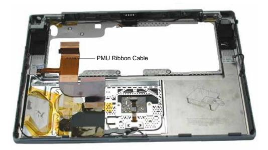
2. Use a black stick to peel off the Kapton tape from the PMU ribbon cable. Reserve the ribbon cable for the replacement top case.
