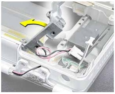
6. Tilt up the inverter board, and disconnect the PMU cable. Lift out the inverter board.
